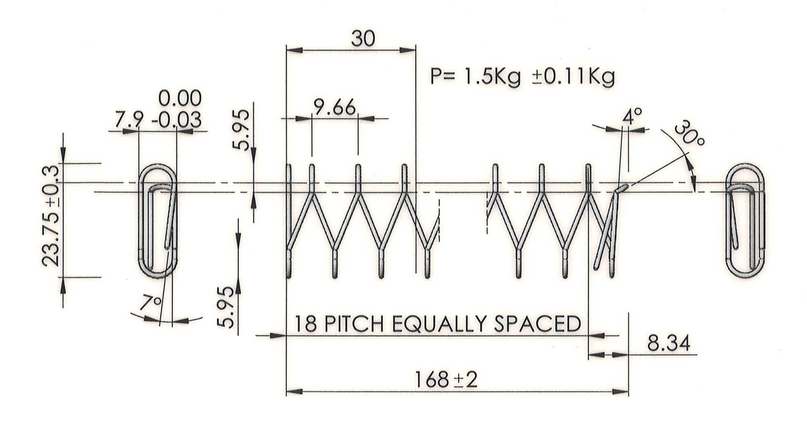
COIL TYPE - LEFT HAND WOUND TOTAL NO. OF COIL - 18 FREE LENGTH - 168 mm ±2 WIRE DIA. - 0.9 mm ±0.015
