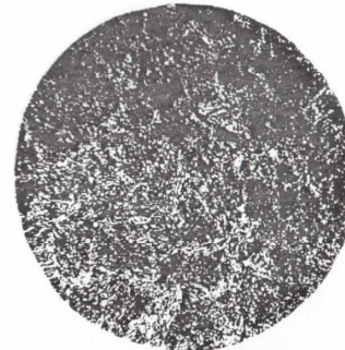
Mark 10 Upper feather like bainite with ferrite along the border of granules
