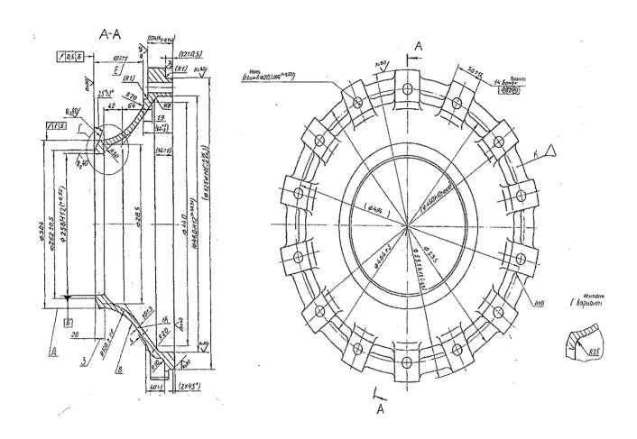
FIG: SLEEVE TO DRG. NO 172.54.002
