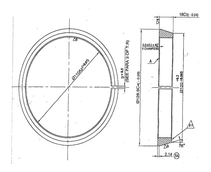
FIG: CONE REAR TO DRG.NO.172.45.008.
