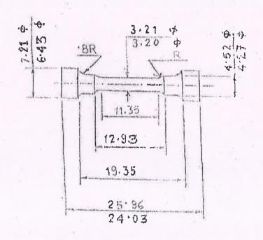
MACHINING FINISH: Ra = V EMERYGRIT 220 FINISH: Ra = 0:36AL DIMENSIONS ARE IN THE MTL. TUNGSTEN ALLOY
