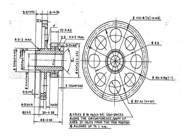
FIG: CLUSTER GEAR TO DRG. NO 172.25.009-1
